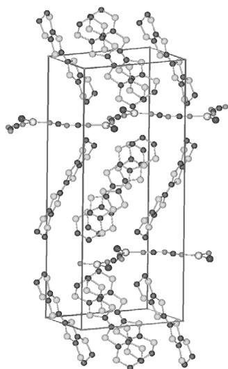
Fig. 1. Crystal structure of  $\kappa$ -(BEDT-TTF) $_2$ X, where X stands for Cu[N(CN) $_2$ ]Br and Cu[N(CN) $_2$ ]Cl.
