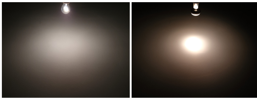
Figure 8.9: Luminous intensity of two incandescent bulbs of the same electrical power and luminous flux, classic isotropic light bulb (left) and reflector light bulb (right). With the reflector light bulb, the light is concentrated into the smaller solid angle, which increases the luminous intensity there. Note that the luminous intensity of the reflector bulb also depends on the deflection angle.
