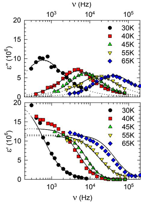
Fig. 5. Imaginary ( $\epsilon''$ ) and real ( $\epsilon'$ ) part of the dielectric function versus frequency for temperature range between 65K and 30K. Full lines are from fits to HN form.
