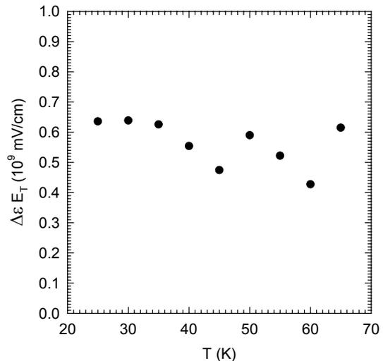
Fig. 7. The product of the oscillator strength and the threshold field.
