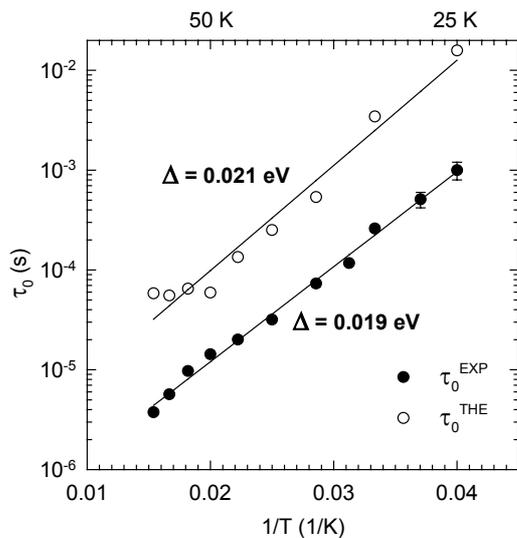
Fig. 6. Experimentally obtained (full dots) and theoretically calculated from non-ohmic contribution data (empty dots) values for relaxation times.
