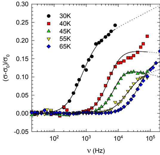
Fig. 4. Real part of the conductivity normalized to the dc value  $((\sigma - \sigma_0)/\sigma_0)$  versus frequency for the temperature range between 65K and 30K. Full lines are fits to HN form.
